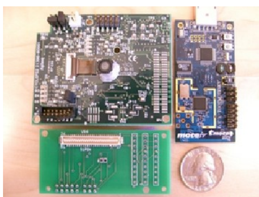
Clockwise from upper left: Cyclops, Tmote, US quarter Coin and Interface Board
